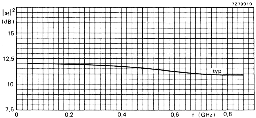
Fig. 4 Transducer gain as a function of frequency; Z_0 = 75 \Omega .
